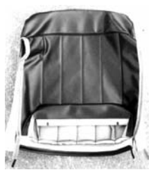
Rear of Front Bucket (Vertical pleats on "plain" vinyl)
